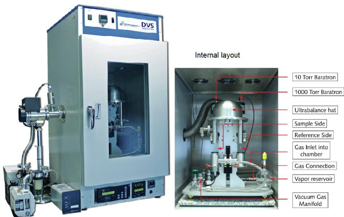
Figure 17 – DVS Vacuum gravimetric sorption analyzer [38]
